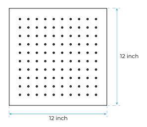
1/2" NPT inlets Easy clean nozzles Flow Rate: 9.5L/min 2.5 GPM
